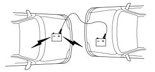
3. Remove the jumper cable from the positive (+) terminal of the booster vehicle's battery.
